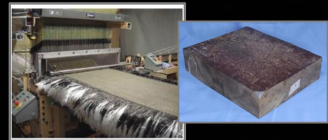
3-D, multi-layer preform weaving technology for thermal protection
