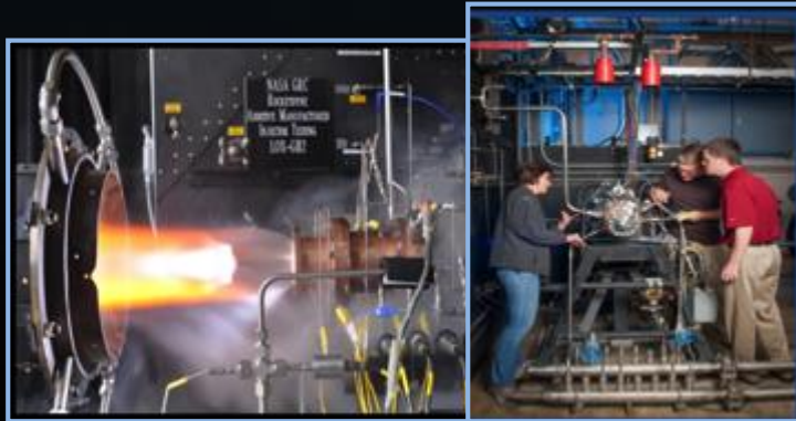
Additive Manufacturing for combustion chambers and nozzles
